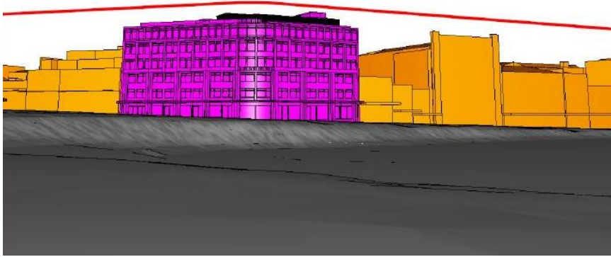
Figure 36: Model view of proposal from within Victoria Park, with line at RL 42 AHD above the street property boundary shown
